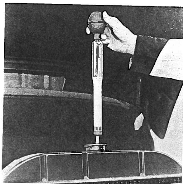
Fig.5a Using an Anti-Freezer Tester to check the strength of the anti-freeze solution
